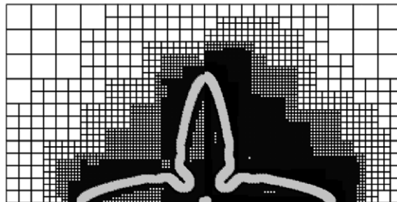
Fig. 2. Adaptive meshes after t = 2000 for C = 1/2 and left E_c = 0.25 and right E_c = 1.00 , the finest mesh is shaded grey.
